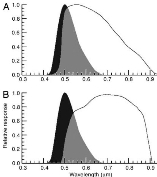
**Fig. 2.** Laboratory emission spectra of bioluminescent bacteria (black area) compared with spectral response functions. Data are shown for the U.S. Defense Meteorological Satellite Program OLS nighttime visible band of the sensor used in this study (A) and the proposed National Polar-orbiting Operational Environmental Satellite System Visible/Infrared Imager/Radiometer Suite day/night band (B). Regions of spectral overlap are shown in gray.
