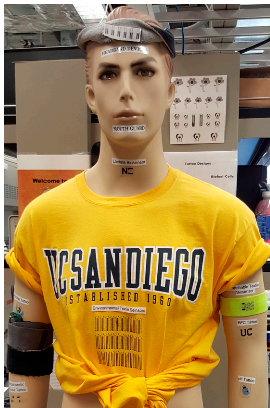
A mannequin in Joseph Wang's laboratory shows off several printed electronic devices, along with a T-shirt, headband, and a swimsuit carrying panels of sensors. The mannequin's arms and collarbone are stuck with electronic tattoos.
