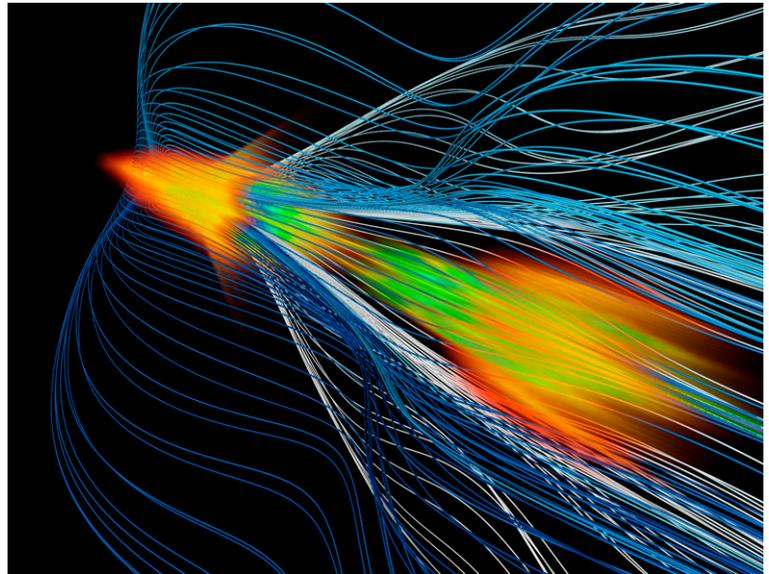
**A new particle collider approach accelerates high-energy positrons in an ionized gas or plasma. Here, a simulation shows the formation of a high-density plasma (green/orange color) around a positron beam moving from the bottom right to the top left. Plasma electrons pass by the positron beam on wave-like trajectories (lines). Image courtesy of Weiming An (University of California, Los Angeles, CA).**
