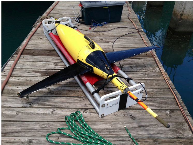
NOAA scientists are developing underwater vehicles, known as gliders, that can record sound and then transmit it back to researchers via satellite. The glider shown here has three microphones, each capable of capturing different frequencies of marine sounds. Image courtesy of Ethan Roth (University of Hawaii at Manoa, Honolulu).
