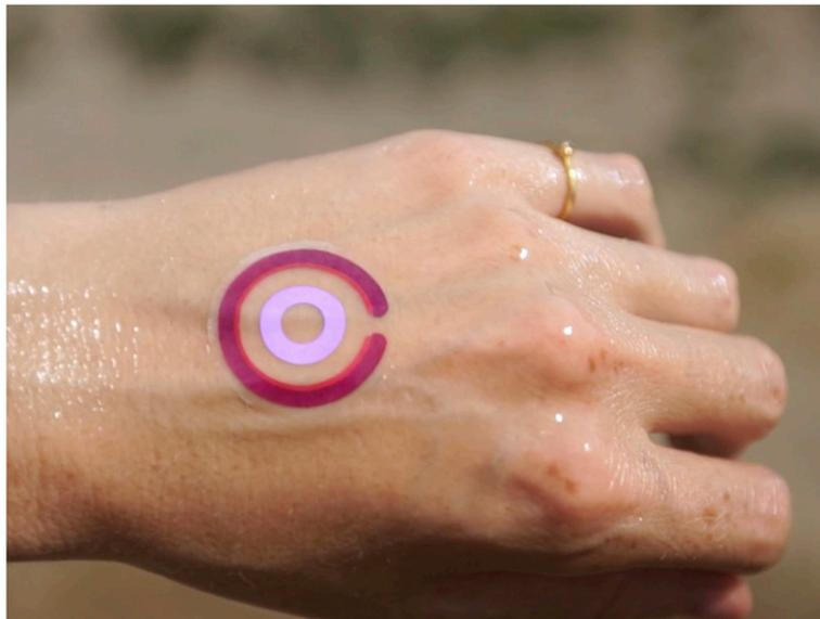
The soon-to-be-released LogicInk UV tattoo will indicate cumulative UV exposure with an outer ring and current UV levels with an inner one. Image courtesy of LogicInk Corporation.
