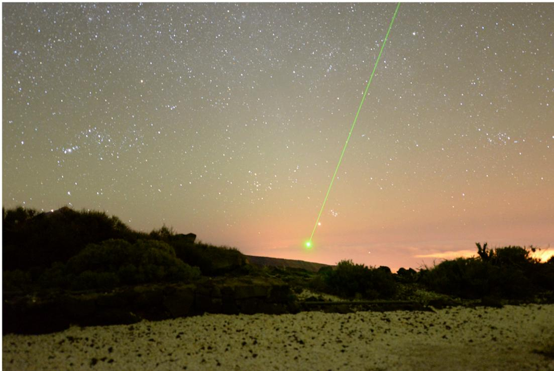
In 2016 researchers used laser light with optical orbital momentum to beam a message a record 143 kilometers between the Canary Islands of La Palma and Tenerife. Image courtesy of Mario Krenn (University of Vienna, Vienna).
