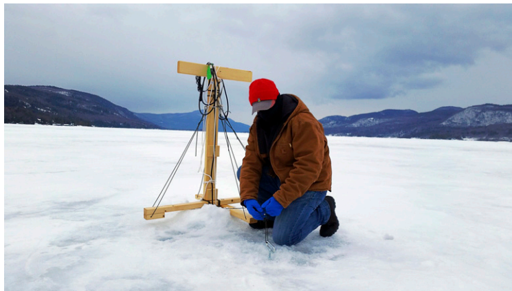
Jefferson project researchers deploy an Acoustic Doppler Current Profiler through the ice to track the direction and speed of the water current. Image courtesy of Rensselaer Polytechnic Institute.
