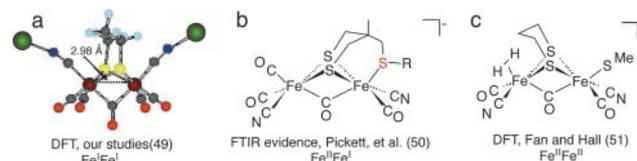
**Fig. 6.** Calculated and observed diiron complexes with a bridging CO group, closer structural analogues to the active site of  $[\text{Fe}]_{\text{H}_2\text{ase}}$ .
