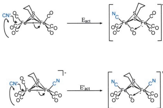
**Fig. 5.** Proposed mechanism for the two-step  $\text{CN}^-/\text{CO}$  substitution reaction in  $(\mu\text{-pdt})[\text{Fe}(\text{CO})_3]_2$  to yield  $(\mu\text{-pdt})[\text{Fe}(\text{CO})_2(\text{CN})]_2^-$ .
