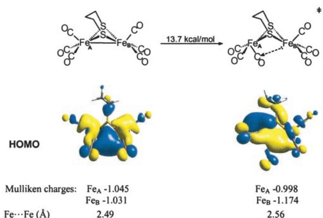
**Fig. 4.** Polarization of Fe—Fe bond electron density upon  $\text{Fe}(\text{CO})_3$  unit rotation in  $(\mu\text{-pdt})[\text{Fe}(\text{CO})_3]_2$  as shown by the highest occupied molecular orbitals (HOMOs) and the Mulliken charges.
