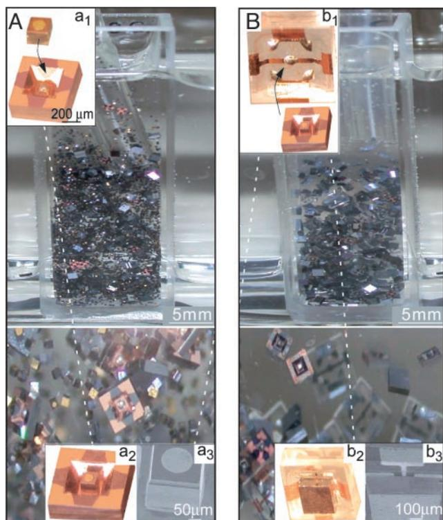
**Fig. 2.** Experimental realization of LED chips that were assembled and packaged by SSSDS. (A and B) Photographs (Upper) and micrographs (Lower) of the chip-on-carrier assembly and chip encapsulation. Insets show device components before ( $a_1$  and  $b_1$ ) and after ( $a_2$  and  $b_2$ ) each assembly step. The scanning electron micrographs ( $a_3$  and  $b_3$ ) illustrate the alignment between components.
