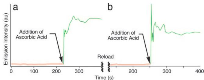
**Fig. 4.** Release of the rhodamine B guest molecules is monitored by following the luminescence intensity of the solution. (a) After the valve has been opened by reduction of the TTF<sup>2+</sup> dication with ascorbic acid, the luminescence in solution increases rapidly. (b) More guest molecules can be loaded into the pores and the valve closed by oxidation of the TTF station and later released by another reduction with ascorbic acid.
