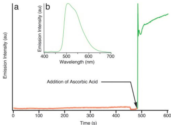
**Fig. 2.** Fluorescence data demonstrating the controlled release of the  $\text{Ir}(\text{ppy})_3$  guest molecules from the nono valve. (a) Release of the  $\text{Ir}(\text{ppy})_3$  molecules from the pores can be monitored by luminescence spectroscopy. When the valve is opened by reduction of the  $\text{TTF}^{2+}$  dication with ascorbic acid, the luminescence of the solution increases rapidly. (b) The visible spectrum of the released  $\text{Ir}(\text{ppy})_3$  molecules is shown.
