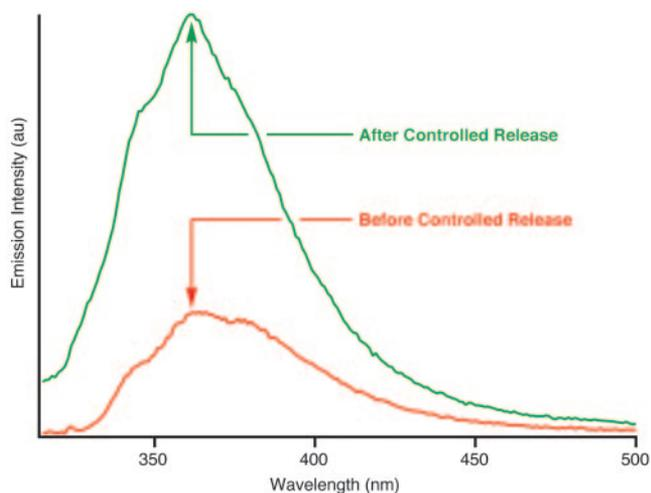
**Fig. 3.** Naphthalene luminescence is used to monitor the operation of the valve. In its closed state when the CBPQT<sup>4+</sup> ring encircles the DNP station, naphthalene luminescence is quenched by the tetracationic cyclophane. When the valve is in its open state when the CBPQT<sup>4+</sup> ring encircles the TTF station, the luminescence intensity of the naphthalene ring system in the DNP station increases 4-fold.
