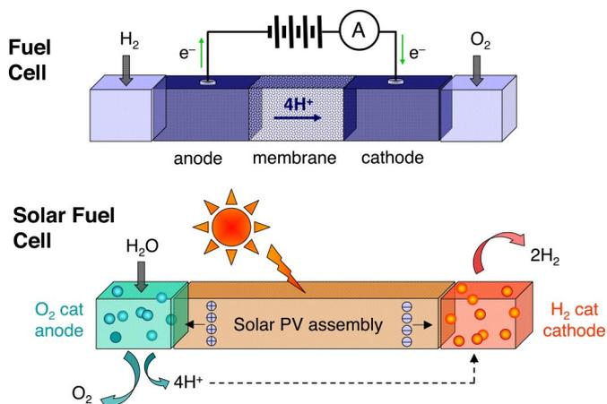
**Fig. 1.**  $\text{H}_2$  and  $\text{O}_2$  are combined in a fuel cell to generate a flow of electrons and protons across a membrane, producing electrical energy. The solar fuel cell uses light to run the electron and proton flow in reverse. Coupling the electrons and protons to catalysts breaks the bonds of water and makes the bonds  $\text{H}_2$  and  $\text{O}_2$  to effect solar fuel production.
