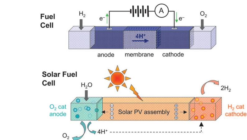
**Fig. 1.**  $\text{H}_2$  and  $\text{O}_2$  are combined in a fuel cell to generate a flow of electrons and protons across a membrane, producing electrical energy. The solar fuel cell uses light to run the electron and proton flow in reverse. Coupling the electrons and protons to catalysts breaks the bonds of water and makes the bonds  $\text{H}_2$  and  $\text{O}_2$  to effect solar fuel production.
