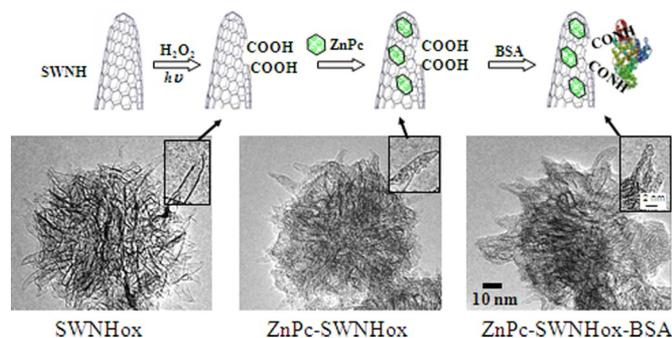
**Fig. 1.** Preparation of ZnPc-SWNHox-BSA. (A) Diagram showing steps in the production of ZnPc-SWNHox-BSA. The nanohorns were visualized by TEM at each stage of production. (B) SWNHox. (C) ZnPc-SWNHox. (D) ZnPc-SWNHox-BSA. (Insets) Magnified images.
