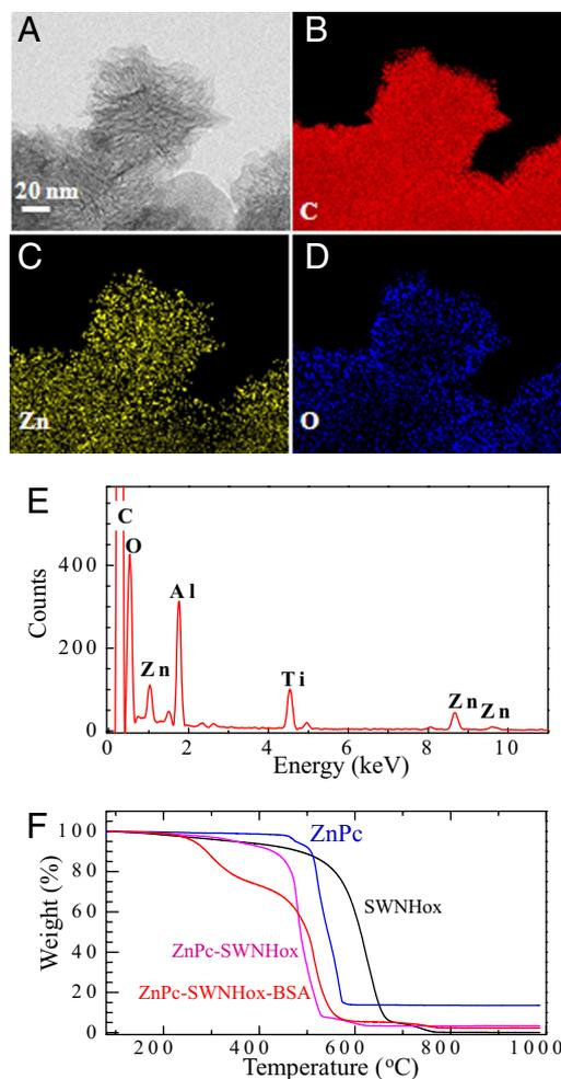
**Fig. 2.** Characterization of ZnPc-SWNHox-BSA by EDX and TGA. (A) Representative STEM image of one aggregate of ZnPc-SWNHox-BSA. (B–D) Atom-mapping images of C (B), Zn (C), and O (D). (E) Representative EDX spectra of ZnPc-SWNHox-BSA. (F) TGA results of SWNHox (black line), ZnPc powder (magenta line), SWNH-BSA (blue line), and ZnPc-SWNHox-BSA (red line).
