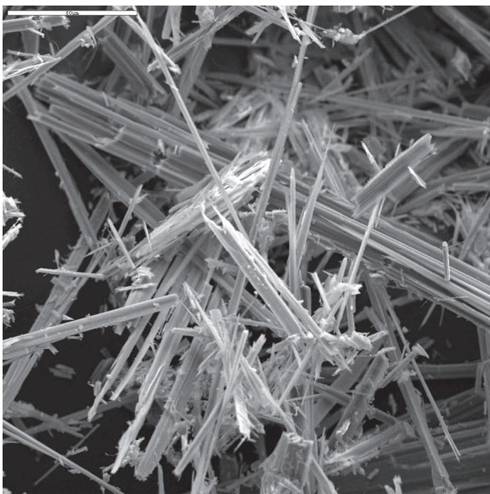
Fig. 1. SEM picture of asbestos fibers (6).
