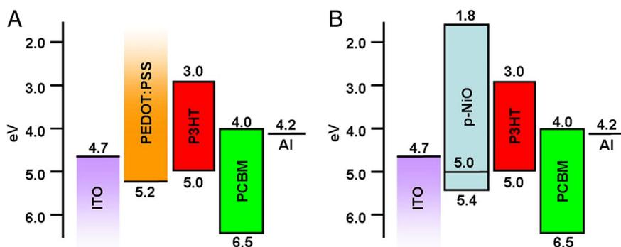
**Fig. 2.** Energy level diagrams of device components referenced to the vacuum level. (A) Typical P3HT:PCBM BHJ OPV with a PEDOT:PSS hole transport layer. (B) Device structure reported here. The published valence band, conduction band, and the Fermi level energies of NiO are shown.
