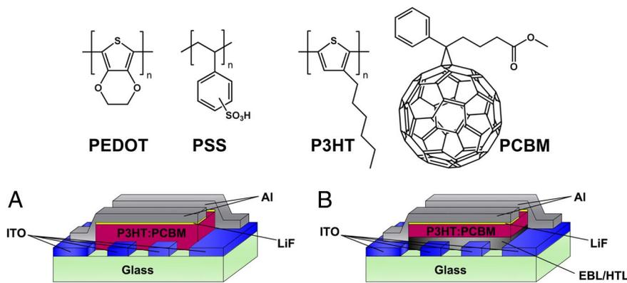
**Fig. 1.** Schematic drawings of the bulk-heterojunction photovoltaic device structures used here without (A) and with (B) an interfacial electron-blocking layer/hole-transporting layer (EBL/HTL). The chemical structures of PEDOT:PSS and the active layer components P3HT and PCBM are also shown.
