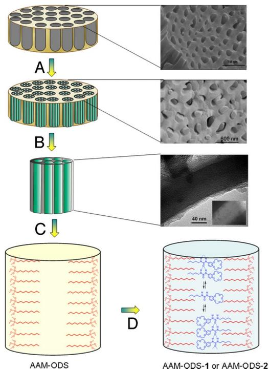
**Fig. 2.** Schematic representation of the synthetic route to obtain functionalized silica mesoporous AAMs filled with mesostructured silica-CTAB (arrow a), then calcinated (arrow b), reacted with hydrophobic ODS (arrow c), and finally filled with the hydrophobic carriers **1** or **2** (arrow d), resulting in the formation of MCM41-ODS-1 and MCM41-ODS-2 materials or of AAM-ODS-1 and AAM-ODS-2 membranes.
