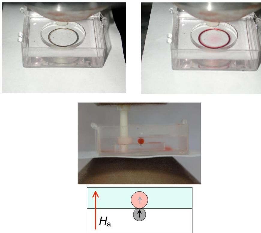
**Fig. 2.** Formation and cross section of paramagnetic liquid tubes. A circular iron track embedded in a Lucite disc, immersed in water and placed in a vertical magnetic field of 0.5 T (Upper Left). When a 1.5 M  $\text{CoCl}_2$  solution is injected near the track it does not disperse, but forms a paramagnetic liquid tube along the track (Upper Right). (Lower) The cross-section of a straight tube of 1 M  $\text{ErCl}_3$  in a vertical field of 1 T.
