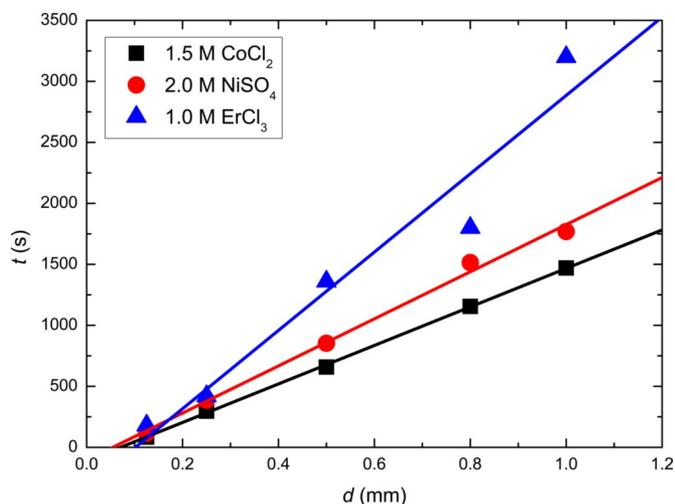
**Fig. 3.** Time taken for a magnetically-confined paramagnetic liquid tube of 1.5 M  $\text{CoCl}_2$ , 2.0 M  $\text{NiSO}_4$ , and 1.0 M  $\text{ErCl}_3$  to diffuse away in water, plotted against the diameter of the iron track,  $d = 2r_i$ .
