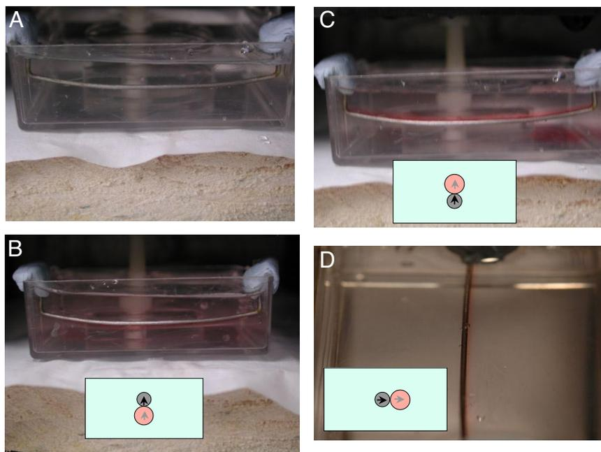
**Fig. 5.** Paramagnetic liquid tubes stabilized by an immersed track. (A) An iron wire immersed in water. (B–D) Stable positions for a paramagnetic liquid tube are above (C) and below (B) the ferromagnetic wire in a vertical field, and at either side of it in a horizontal field (D). The photographs show tubes of  $\text{ErCl}_3$  in water.
