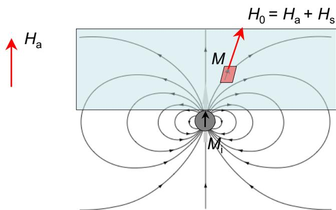
**Fig. 1.** The different magnetic fields and magnetizations involved in the experiments.  $M$  is the magnetization of an element of liquid,  $M_i$  is the magnetization of the iron track,  $H_a$  is the uniform field applied by using a permanent magnet or an electromagnet,  $H_s$  is the stray field created by  $M_i$ , and  $H_0 = H_a + H_s$  is the magnetic field acting on  $M$ . The demagnetizing field  $H_d$  is very small in  $M$ , but not in  $M_i$ .
