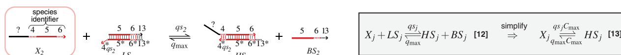
Fig. 4. Buffering module: DNA implementation of the buffering module used to cancel out the buffering effect. A buffering module is needed for each formal species X_j for which \sigma_j < \sigma . The buffering module for species X_2 is shown. X_2 reversibly displaces BS_2 from complex LS_2 to produce complex HS_2 similarly to the first reaction of the bimolecular module. The black domain (13) is unique to this buffering module for species X_2 . Set qs_j = \gamma^{-1}(\sigma - \sigma_j) . Reaction equations 12 are used in simulations (Figs. 5 and 6); simplified reaction equations 13 are useful for analysis.
