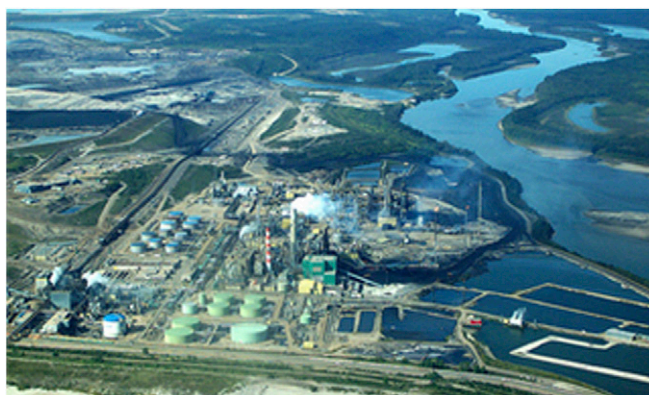
Fig. 1. Aerial view of an oil sands extraction facility with adjacent OSPW holding ponds and the Athabasca River. Companies currently operate under a no-release strategy, so all OSPW must be stored in containment ponds to prevent release into the environment. The Athabasca River is the main source of fresh water used in the bitumen extraction process. (Copyright © The Pembina Institute, Calgary, Alberta, Canada. Photograph courtesy of Chris Evans, The Pembina Institute, www.OilSandsWatch.org.)
