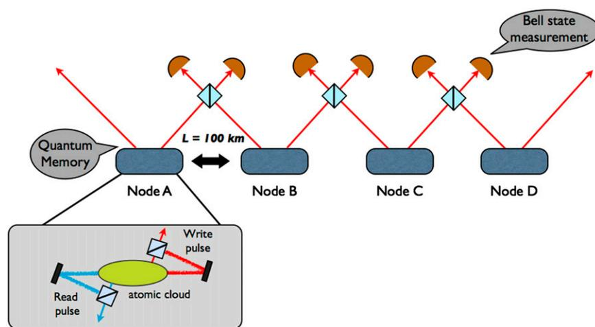
**Fig. 1.** Sketch of a future quantum communication network expanding over long distances. Each quantum memory consisting of an atomic cloud lies within a node of the network. Quantum states are teleported from one node to another by performing Bell state measurements. (Inset) Write and read pulses used to create the entanglement between the atomic ensemble and the write-out photon.  $L$  corresponds to the length of the communication channel between two adjacent nodes.
