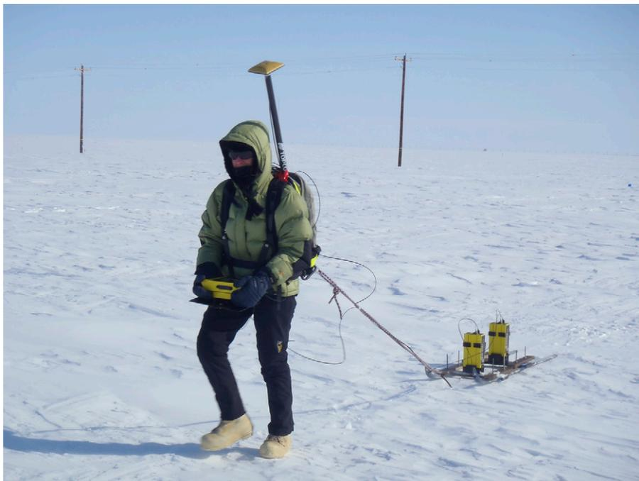
Susan Hubbard tugs a ground-penetrating radar device attached to skis across the Arctic permafrost to get measurements of the frozen ground below. Image courtesy of Susan Hubbard.
