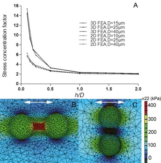
**Fig. 2.** (A) 3D FEA results of stress concentration factor calculated for the area between two particles located along the tensile axis in a fibrous cap. Stress concentration factor rises exponentially when the distance between the two spherical  $\mu\text{Calcs}$  decreases. Results are compared with previous 2D FEA reported in the work by Maldonado et al. (10). B and C show FEA results for particles with initial  $h/D = 0.4$  oriented along and transverse the tensile axis, respectively.
