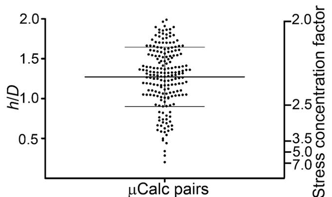
**Fig. 3.** Ratio  $h/D$  for 193 pairs of  $\mu\text{Calcs}$  embedded in fibrous caps where  $h/D < 2$  and the corresponding stress concentration factor when embedded in a fibrous cap along the tensile axis. Lines indicate mean  $\pm$  SD.
