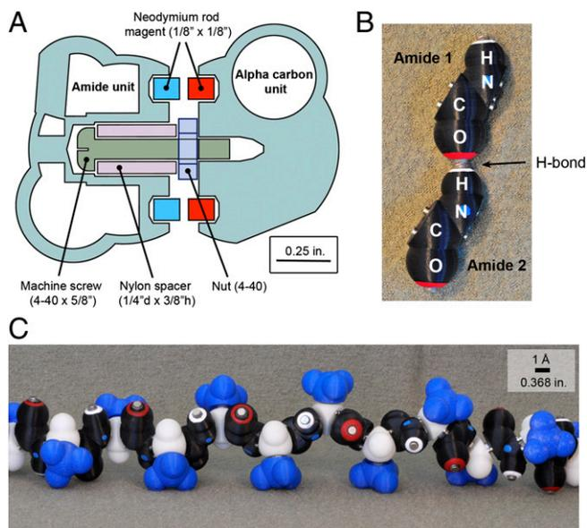
**Fig. 5.** Peppytide model assembly. (A) Bore dimensions and assembly plan for the amide unit and  $\alpha$ -carbon unit joint (cross-section view drawn to scale); the same scheme was used for the  $C_{\alpha}$ - $CH_3$  joint. (B) Representation of a hydrogen bond between distal amides. (C) A Peppytide homopolymer (polyalanine); black part, amide unit; white part,  $C_{\alpha}$  unit; blue part, methyl group unit; red ring, oxygen; white ring, hydrogen; blue dot, nitrogen.
