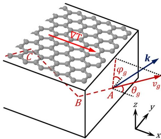
**Fig. 5.** Schematic used to derive the phonon-boundary scattering model in a MLG ribbon where the group velocity and wave vector are not collinear because of the highly anisotropic structure. In this schematic,  $\theta$  and  $\varphi$  are the polar angle with  $x$ -axis and the corresponding azimuthal angle in the  $yz$ -plane, respectively. The subscript  $g$  is used to denote the group velocity.
