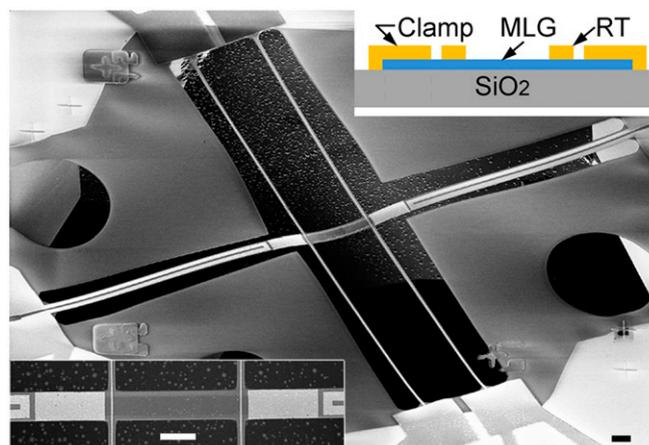
**Fig. 1.** Scanning electron micrograph of the MLG sample G34 at a 45° view angle. The top and bottom insets show schematic cross-section and top view of the central bridge, respectively. (Scale bar, 10  $\mu$ m.)
