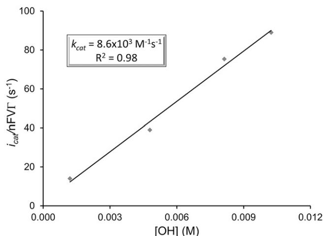
Fig. 5. Variation of  $i_{cat}$  normalized for surface coverage with  $[\text{OH}^-]$  in 0.25 M  $\text{LiClO}_4$  with  $[\text{PO}_4^{3-}] = 12\text{mM}$ . The  $i_{cat}$  values at 1.6 V were obtained by Tafel extrapolation; see text and Fig. S6 for details.
