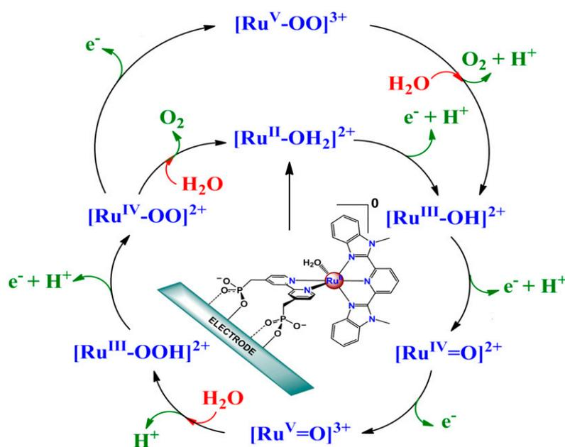
**Fig. 2.** Water oxidation mechanism for *nanoITO*- $\text{Ru-OH}_2^{2+}$ .
