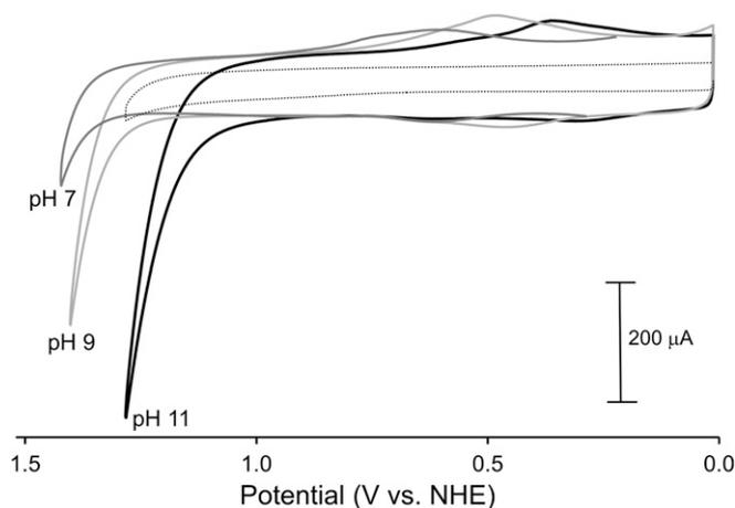
**Fig. 4.** CVs for 1-ALD at  $23 \text{ }^\circ\text{C}$  and 20 mV/s in  $I = 0.1 \text{ M}$  of the added buffers at pH values indicated in figure. The dashed line is the background current at pH 11.1 from a  $\text{nanoITO}$  electrode with 20 ALD cycles of  $\text{TiO}_2$  and no catalyst loading.
