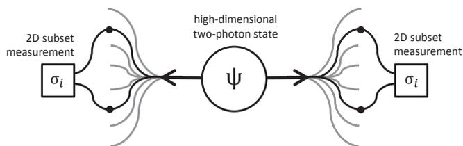
**Fig. 1.** Visualization of the measurement concept. The two photons are sent in two different directions. Each of the photons is in a mixture of many modes. We perform the same two-dimensional subspace measurement on both photons. When we consider all two-dimensional subspaces, we can determine the dimensionality of entanglement.
