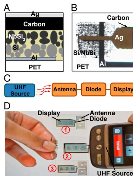
**Fig. 1.** (A) Cross-section of the diode rectifier used by Sani et al. (8). (B) Optical image of the printed diode with the materials components highlighted. (C) Schematic representation of the wireless system powering the e-label display. (D) Picture of the complete antenna-diode-display device and a mobile phone as an RF source. The picture also shows the display switching from the off state (1), to partial (2), and full-on state (3) upon making a phone call.
