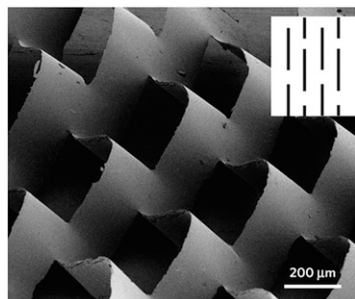
Nanocomposite materials, here made of graphene oxide and polyvinyl alcohol, are cut following kirigami techniques to allow for elasticity and expand functionality. The insets show the corresponding kirigami cuts. Adapted from ref. 1, with permission from Macmillan Publishers Ltd: Nature Materials , copyright (2015).
