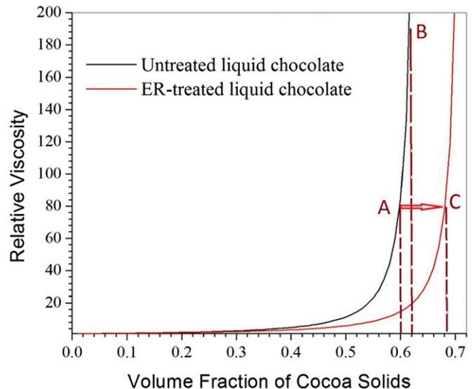
**Fig. 2.** Viscosity of original liquid chocolate and the viscosity of ER-treated liquid chocolate along the flow direction. Point A represents the original state at  $\phi = 0.6$ . Without the ER treatment, removing a small amount of fat leads to dramatically increased viscosity (point B). With the ER treatment, the fat can be reduced by 20% and the viscosity remains the same (point C).
