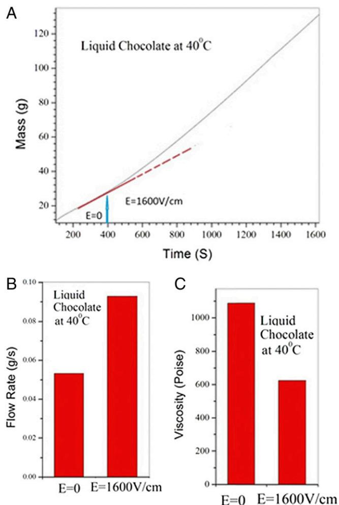
**Fig. 5.** (A) Application of 1,600-V/cm electric field significantly increases the flow rate. (B) The flow rate was increased by 74.3%. (C) The viscosity was reduced by 43.5%.
