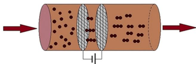
**Fig. 3.** As the liquid chocolate flow passes a strong local electric field, the solid particles aggregate along the field direction to form streamline aggregates and the viscosity along the flow direction is significantly reduced.
