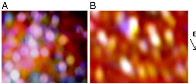
**Fig. 1.** Under microscope, (A) the original cocoa solids in liquid chocolate are spherical around 2  $\mu\text{m}$ ; (B) the electric field aggregates these particles into short chains, which are similar to prolate spheroids.
