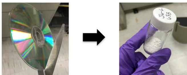
**Fig. 4.** Repurposing a compact disk as a monomer source for the depolymerization of PC and repolymerization to PSU. Compact disk (left) and PSU powder (right) are shown before and after the depolymerization/repolymerization process.
