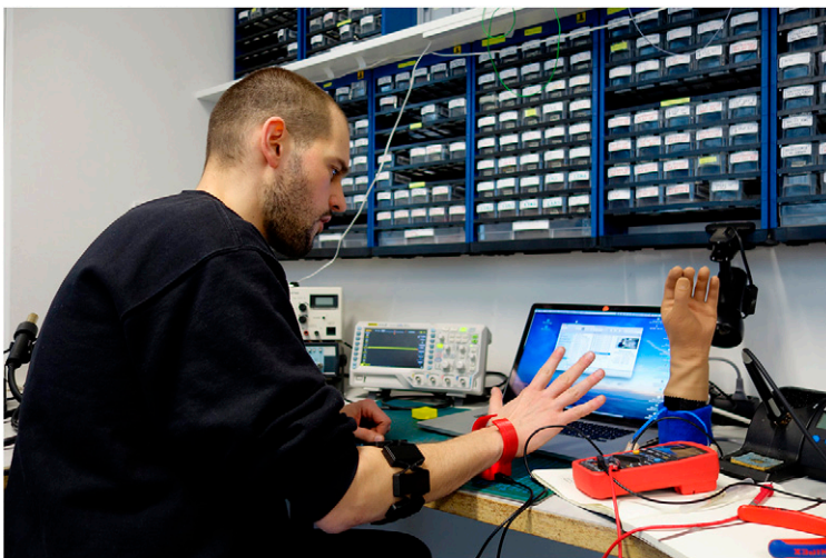
Master’s student Maximilian Mahal, working at Fab Lab in Berlin, tries out a prototype prosthetic-aid for computer users, called Shortcut, which employs wireless signals from amputee limbs to manipulate computer applications. Image courtesy of Lucas Rex, David Kaltenbach, and Maximilian Mahal.
