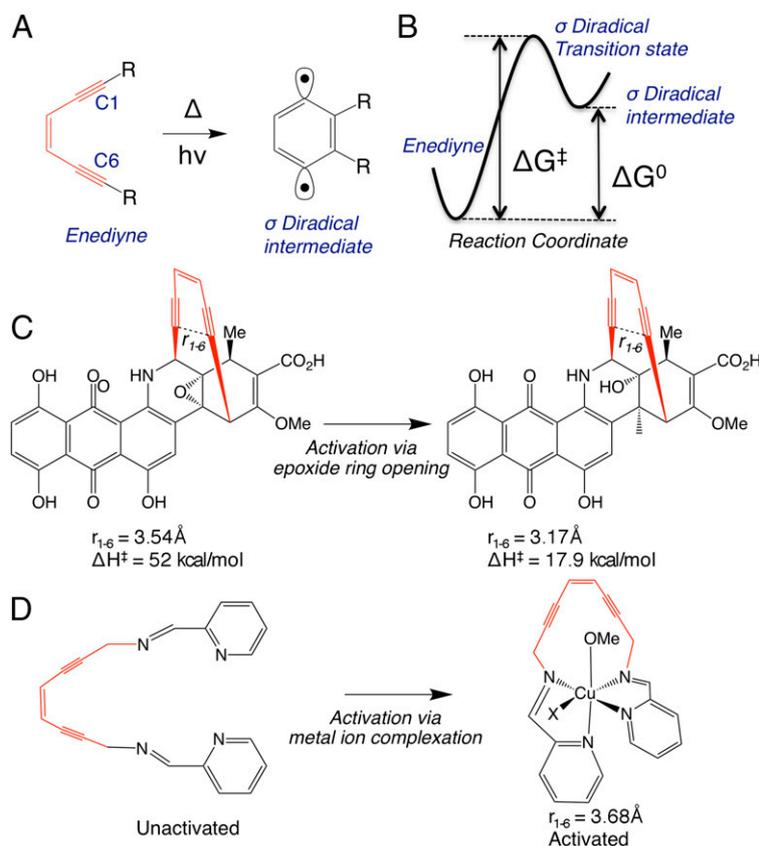
**Fig. 1. (A)** Thermal and photochemical activation of enediynes to the diradical intermediate. **(B)** Simple potential energy diagram indicating the intermediate nature of the diradical. **(C)** Activation of dynemicin A via epoxide ring opening. **(D)** Activation of the PyED ligand by metal ion complexation. In C and D, the enediyne warhead is depicted in red.
