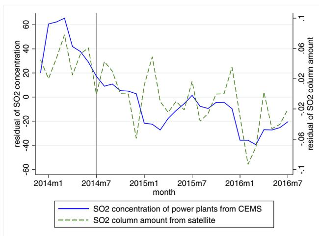
**Fig. 2.** Demeaned SO<sub>2</sub> concentrations from CEMS on power plants with capacity above 1,000 MW versus SO<sub>2</sub> column amounts from satellite observations in surrounding areas.
