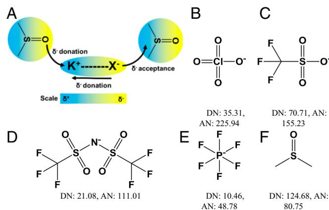
**Fig. 1.** (A) Schematic representation of the solvent–salt ( $KX$  where  $X$  is the anion) interactions in the electrolyte (the charge distributions are only illustrative and do not represent actual electron density or distribution) and chemical structures of the potassium salt anions investigated: (B) perchlorate, (C) trifluoromethanesulfonate, (D) bis(trifluoromethanesulfonyl)imide, (E) hexafluorophosphate, and the solvent (F) DMSO.
