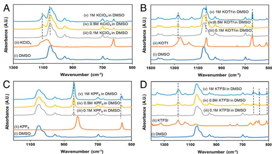
**Fig. 3.** FTIR spectra of the electrolytes used in this study with various salt concentrations: (A)  $\text{ClO}_4^-$  anion, (B)  $\text{OTf}^-$  anion, (C)  $\text{PF}_6^-$  anion, and (D)  $\text{TFSI}^-$  anion.
