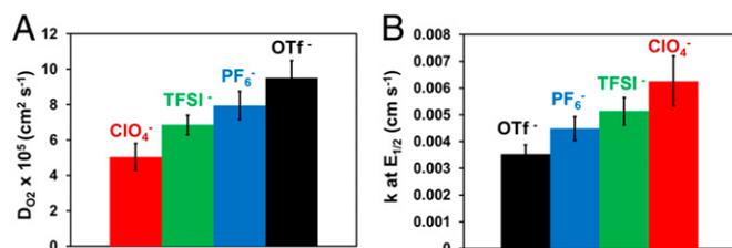
**Fig. 4.** The impact of the salt anion on the (A) diffusion coefficient of O<sub>2</sub> and (B) ORR rate constants at the half-wave potential (E<sub>1/2</sub>). The diffusion coefficients were calculated using the N-S equation (CVs in *SI Appendix, Fig. S4*). The ORR rate constants were calculated using the K-L equation (LSVs in *SI Appendix, Fig. S6*). The error bars were calculated from at least 3 independent measurements.
