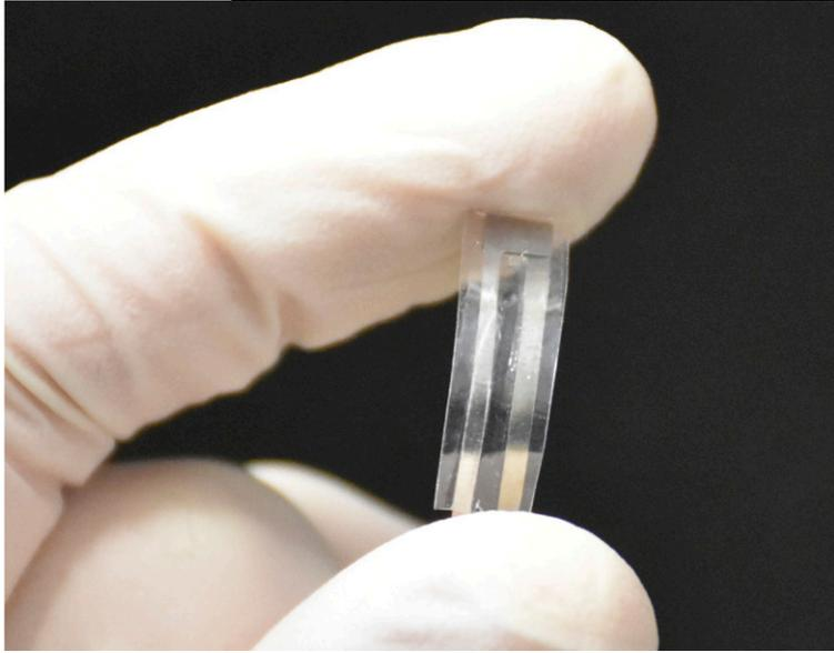
**A sensor made from a biodegradable polymer detects the force of breathing movements when placed on a mouse's diaphragm. Less invasive than a catheter-based sensor, it dissolves on its own and doesn't need to be removed—making it potentially useful for monitoring patients who undergo anesthesia. Image credit: Thanh Nguyen (University of Connecticut, Storrs, CT).**
