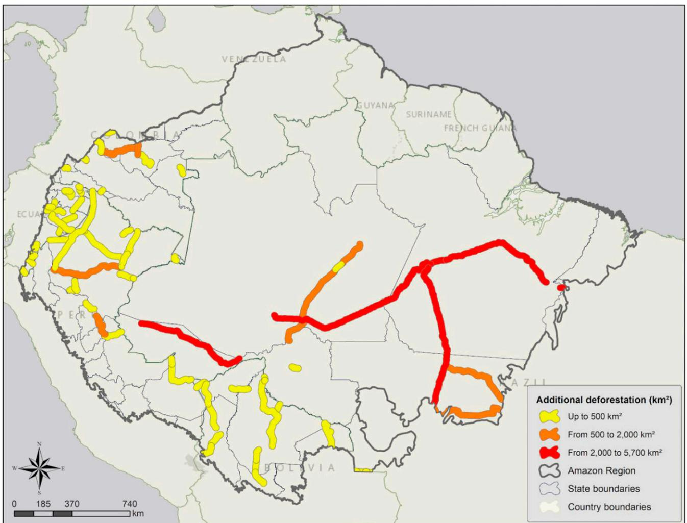
**Fig. 1.** Predicted deforestation in the 20-km buffer around selected road projects (20 y). Using historical data on tree cover loss and a spatial simulator software (DinamicaEGO), we estimated the deforestation that would be caused by each road project as the difference between predicted deforestation with and without implementation of the road. The countries are in beige and their boundaries are in gray/olive.
