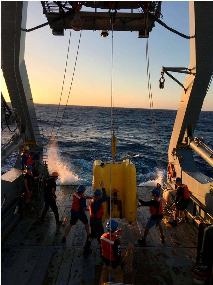
The Clio autonomous underwater vehicle, or AUV, is already unlocking secrets of the ocean's microbial and chemical composition. The AUV's unusual shape is streamlined for vertical motion through the water column. Image credit: Mak Saito (Woods Hole Oceanographic Institution, Woods Hole, MA).
