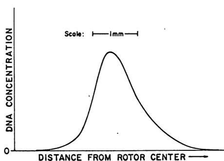
FIG. 4.—The concentration distribution of calf thymus DNA banded in cesium chloride. 2.7  $\mu$ g. of calf thymus DNA (prepared by a detergent method by Dr. C. Jardetzky) was centrifuged at 44,700 rpm in 7.7 molal cesium chloride at pH 8.4. The skewness in the resultant band indicates heterogeneity in effective density.
