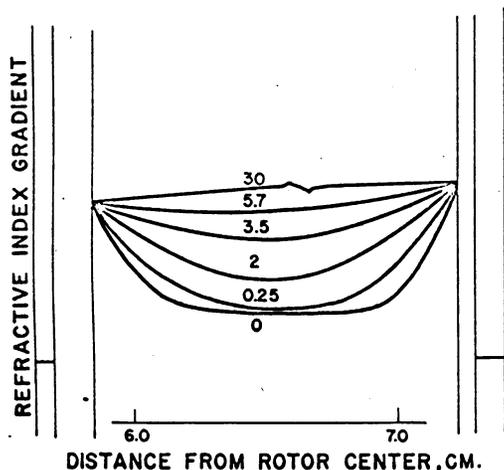
FIG. 1.—Superimposed schlieren diagrams of successive stages in the development of a cesium chloride equilibrium gradient. The numbers above each curve are the times in hours that the centrifuge has been running at 31,410 rpm. These diagrams are from an experiment in which 8  $\mu\text{g}$ . of DNA was present in the cell; the banded DNA produces a diphasic pip in the final schlieren diagram.
