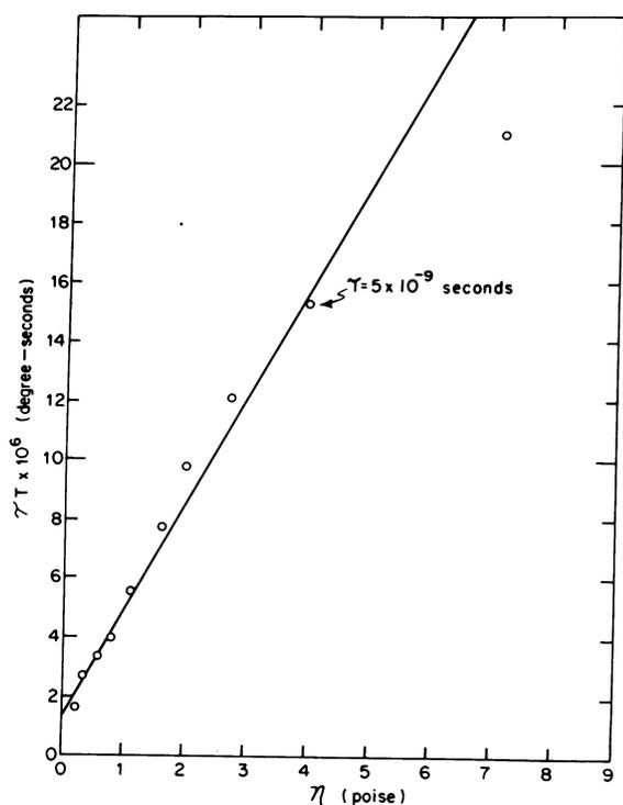
FIG. 1. The relationship between rotational correlation time ( $\tau$ ) calculated by Eq. 1 and the coefficient of viscosity ( $\eta$ ) of the solvent at the temperature of measurement ( $T$ ). Rotational correlation times for methyl-12-nitroxylstearate in castor oil obey Eq. 2, for values of  $\tau$  equal to or less than 5 nsec.
