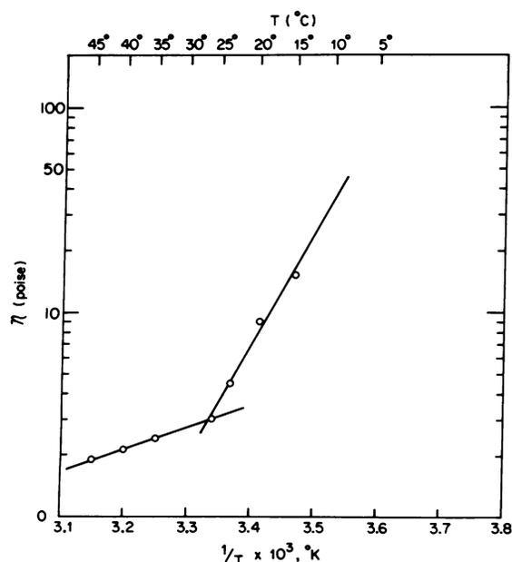
FIG. 3. A phase transition in an *E. coli* phospholipid extract. Lipids were extracted from cells grown at 43° and gave a phase transition at approximately 27°. Viscosities were determined as described in the text.
