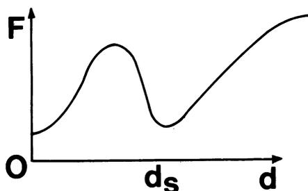
FIG. 1. Free energy as a function of the separation of a positive and negative charge.  $d = 0$  corresponds to a chemical bond and  $d_s$  to the separated charges.
