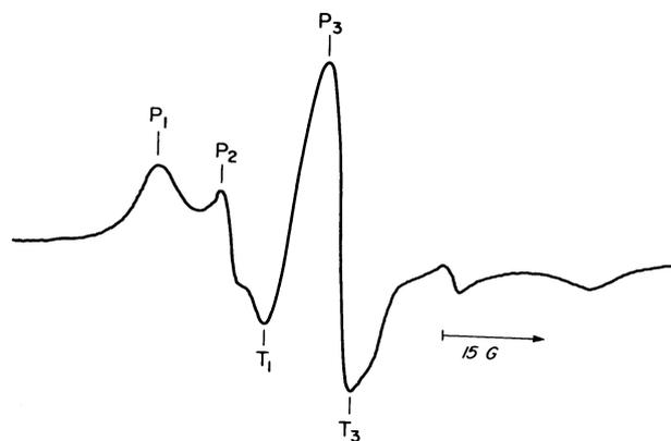
FIG. 1. EPR spectrum of SR labeled with 4 moles of "NEM spin label"/ $10^6$  g. SR is 6 mg/ml in 0.1 M KCl, 5 mM Tris-maleate (pH 7.0), room temperature. Field set, 3385 G; scan range, 100 G. P, peak; T, trough.
