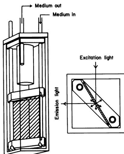
FIG. 1. Device used to hold coverslip in fluorescence cell in the spectrofluorometer. The coverslip (cross-hatched) is aligned at  $30^\circ$  to the excitation beam to minimize the effect of light reflections. Approximately  $30 \text{ mm}^2$  of the coverslip is illuminated (about  $10^5$  cells).
