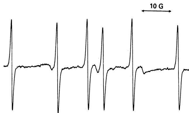
FIG. 6. EPR spectrum of MNPOL-H obtained by allowing MNPOL to react with rat liver microsomes and NADPH. The identical EPR spectrum was obtained by carefully titrating MNPOL with sodium borohydride and oxygen. A_N = 15.7 G; and A_H = 26.2 G. There is also a second species exhibiting a three-line spectrum with A_N = 16 G. This species is most likely due to the dimerization of MNPOL.
