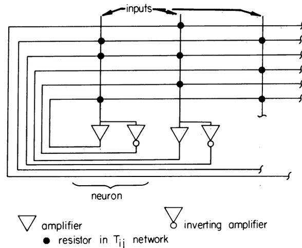
FIG. 2. An electrical circuit that corresponds to Eq. 5 when the amplifiers are fast. The input capacitance and resistances are not drawn. A particularly simple special case can have all positive  $T_{ij}$  of the same strength and no negative  $T_{ij}$  and replaces the array of negative wires with a single negative feedback amplifier sending a common output to each “neuron.”
