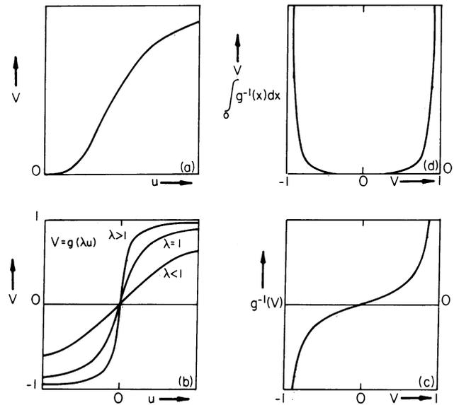
FIG. 1. (a) The sigmoid input–output relation for a typical neuron. All the  $g(u)$  of this paper have such a form, with possible horizontal and vertical translations. (b) The input–output relation  $g(\lambda u)$  for the “neurons” of the continuous model for three values of the gain scaling parameter  $\lambda$ . (c) The output–input relation  $u = g^{-1}(V)$  for the  $g$  shown in b. (d) The contribution of  $g$  to the energy of Eq. 5 as a function of  $V$ .
