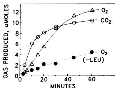
FIG. 2. Production of CO<sub>2</sub> and O<sub>2</sub> during the Mn(II)-dependent decomposition of H<sub>2</sub>O<sub>2</sub> in the presence or absence of leucine. Reactions were carried out in a Warburg apparatus as described in the legend to Table 1. The mixtures (2.0 ml) contained initially 50  $\mu\text{M}$  Mn(II), 23.5 mM NaHCO<sub>3</sub>, 30 mM H<sub>2</sub>O<sub>2</sub>, and either 50 mM (open symbols) or 0 mM (closed symbols) leucine.
