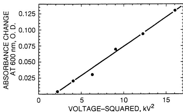
FIG. 3. The amplitude of the electroabsorption spectrum for an oriented D85N film of peak absorbance  $A_{600} = 0.6$ , dried over  $P_2O_5$ , is plotted as a function of the square of the applied voltage. In this series of measurements, the cytoplasmic side of the film was held positive. The dependence on applied voltage is seen to be quadratic, with a threshold.
