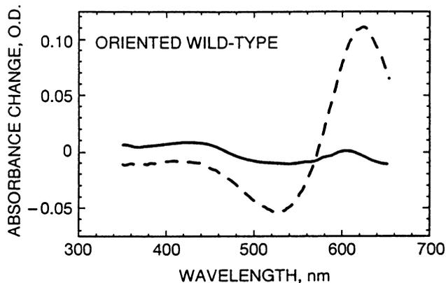
FIG. 1. Electroabsorption spectra recorded for an oriented wild-type BR film of peak absorbance  $A_{560} = 1.2$ , equilibrated at 12% relative humidity, at applied potentials of  $\pm 4000$  V. Dashed line, cytoplasmic side negative; solid line, cytoplasmic side positive. In this and subsequent spectra, noise has been reduced by using smoothed, parabolic B-spline fits.
