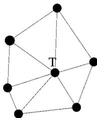
FIG. 4. Acute triangulation around center grid point.
