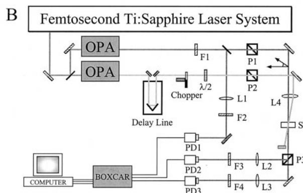
**Fig. 2.** (A) Absorption spectra of the molecules studied. (B) Experimental layout of femtosecond transient absorption apparatus. OPA, optical parametric amplifier; F, optical filters; P, prism polarizers;  $\lambda/2$ , half-wave plate; L, lens; PD, photodiode; S, sample cell.
