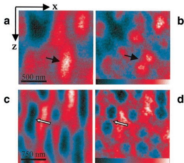
**Fig. 3.** XZ-images of 100-nm-diameter fluorescent beads (a and b) and of 100-nm-diameter negatively stained glass beads agglomerations (c and d) as observed in the confocal (a and c) and the STED-fluorescence (b and d) microscope. Note the artifacts indicated by arrows induced by the elongated spot in the confocal image and their reduction in the STED counterpart.
