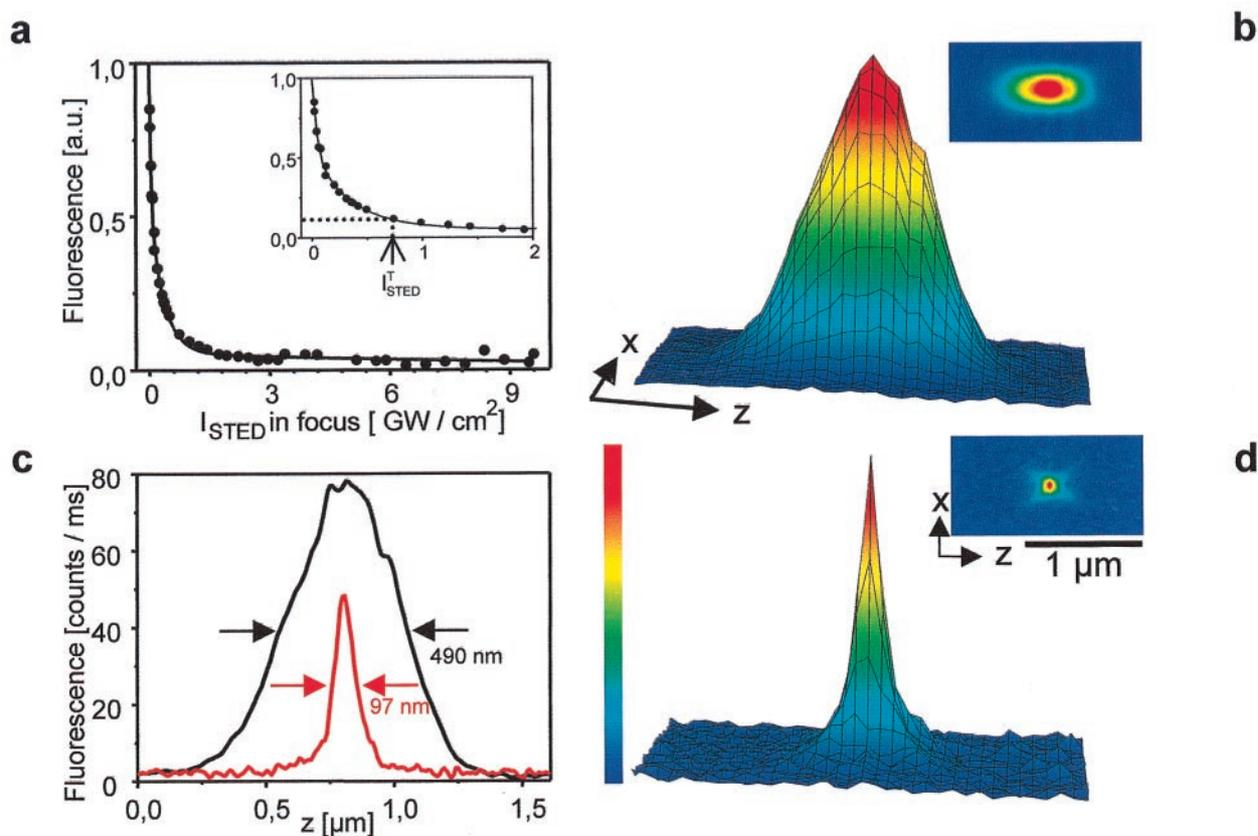
**Fig. 2.** (a) Fluorescence is a nonlinear function of stimulating intensity; 10% remaining fluorescence is obtained for  $I_{\text{STED}}$  corresponding to  $P_{\text{STED}}$  of 2.2 mW in the focus. (b) Surface plot of XZ-section (*Inset*) of confocal fluorescence spot for 1.4 oil immersion lens. (d) Same as b but with STED-beam PSF switched on. (c) Corresponding axial intensity profiles demonstrate 5.1-fold reduction of the axial width (FWHM) from 490 nm down to 97 nm.
