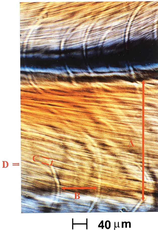
**Fig. 3.** On the ground, self-organization also occurs over smaller distance scales. This photograph is taken from a sample prepared in the laboratory and placed between crossed circular polarizers. In addition to the periodicity of about  $400\ \mu\text{m}$  (A), it also shows periodicities of about  $100\ \mu\text{m}$  (B),  $20\ \mu\text{m}$  (C), and  $5\ \mu\text{m}$  (D). These levels of self-organization did not arise for samples assembled under low  $g$  conditions.
