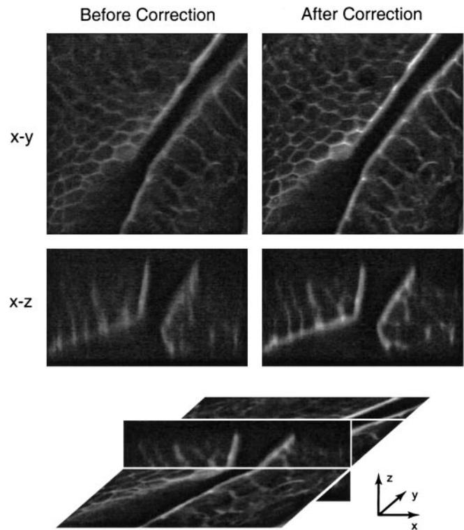
**Fig. 3.** Confocal microscope scans before and after aberration correction.  $x$ - $y$  (lateral) and  $x$ - $z$  (axial) scans of a fluorescently labeled section of mouse intestine specimen are shown. The schematic beneath illustrates the relative three-dimensional orientation of the  $x$ - $y$  and  $x$ - $z$  scans. The image dimensions in the  $x$  and  $y$  directions are 80  $\mu\text{m}$ ; the  $z$  dimension is 15  $\mu\text{m}$ .
